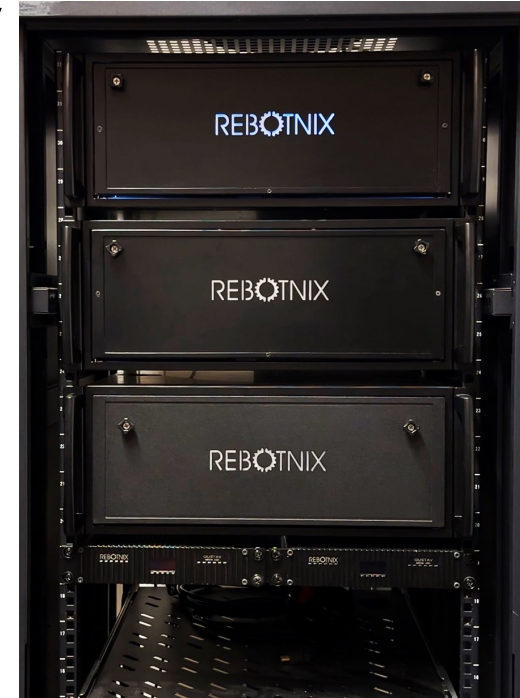
Example of Optimus GPU rack. 196608 GPU CURES, 288 Gigabytes RAM.
